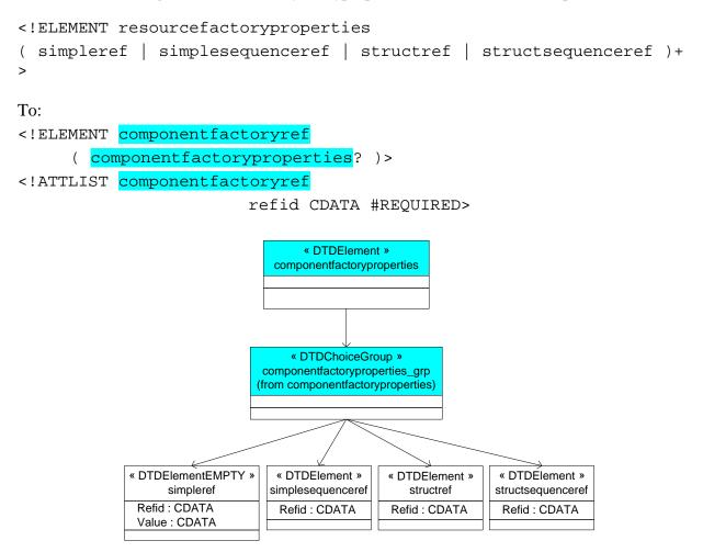
Figure D-26. *componentfactoryproperties* Element Relationships
