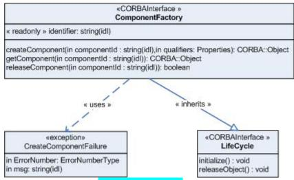
Figure 3-9: *ComponentFactory* Interface UML
